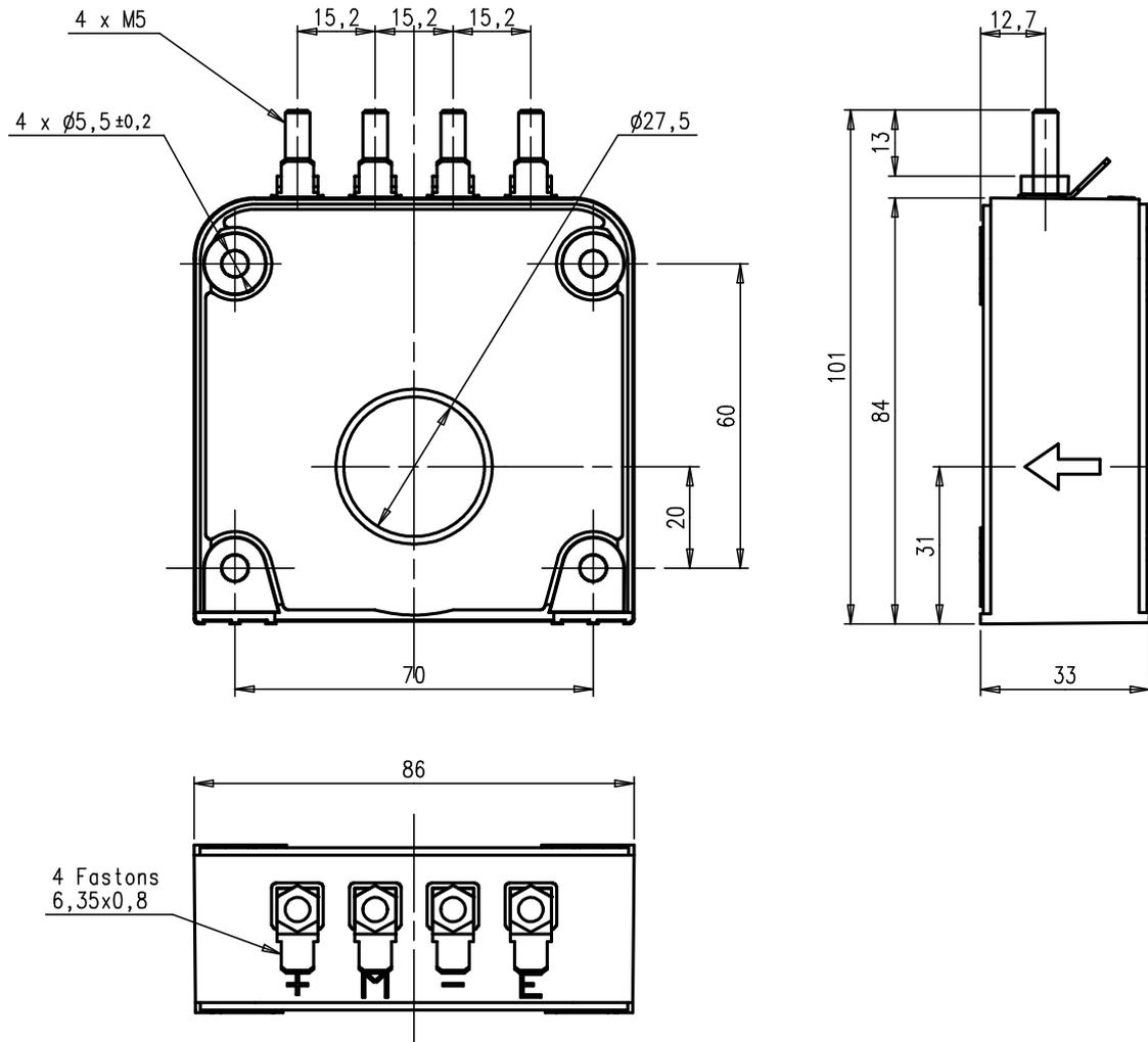
**Maximum M5 tightening torque: 2 N.m**
